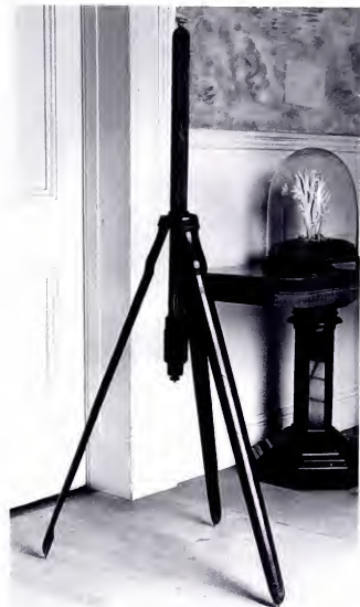
FIGURE 20. Portable Barometer. Belonging to Henry Cavendish. The ingenious case opens into a tripod. Alongside the (now broken) barometer are two scales, one English and one French. There is a thermometer at the bottom with a correction scale. Cavendish may have used this instrument on his journeys outside London. Photograph by the authors. Devonshire Collection, Chatsworth. Reproduced by permission of the Chatsworth Settlement Trustees.
